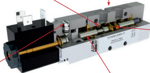
Spacer cages in brass. Unlike the plastic, brass ones do not deform with the change of temperature, giving more stability to the seals and avoiding any possible backlash.
