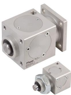
The patented Airwork rod-lock BS series is a mechanical device designed to be used with all ISO 15552 and 6432 VDMA cylinders, and its purpose is to block the rod of the cylinder in any position. This solution allows to block the stroke of the cylinder every time an unexpected fall of pressure takes place. The blocking force is always bigger than the one developed from the corresponding cylinder at 10 bars.
